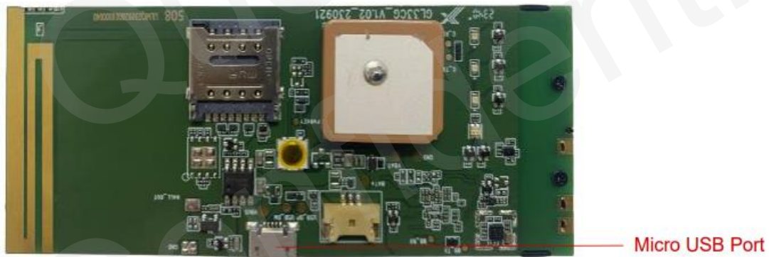
Figure 6. Typical Power Connection
