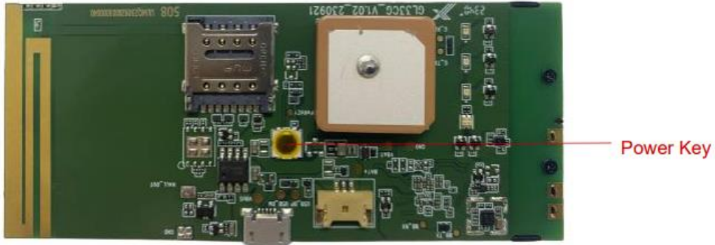
Figure 7. Power On GL33CG
