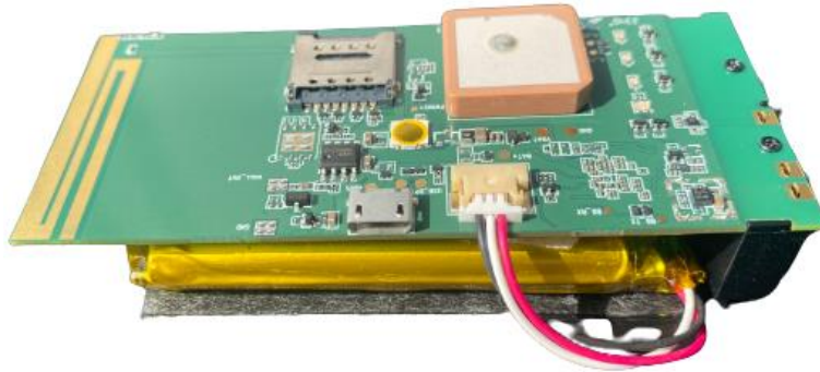
Figure 5. Backup Battery Installation
